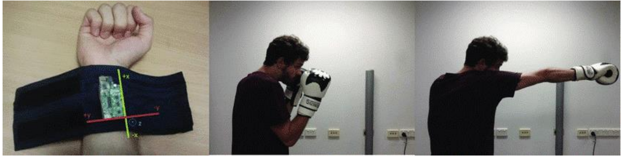
Slika 4. Mjerenje brzine udarca šakom - Scientific Figure on ResearchGate. Preuzeto s: https://www.researchgate.net/figure/The-acceleration-sensor-is-fixed-to-the-inside-of-the-wrist-with-a-velco-band-The-boxing_fig3_282553007
