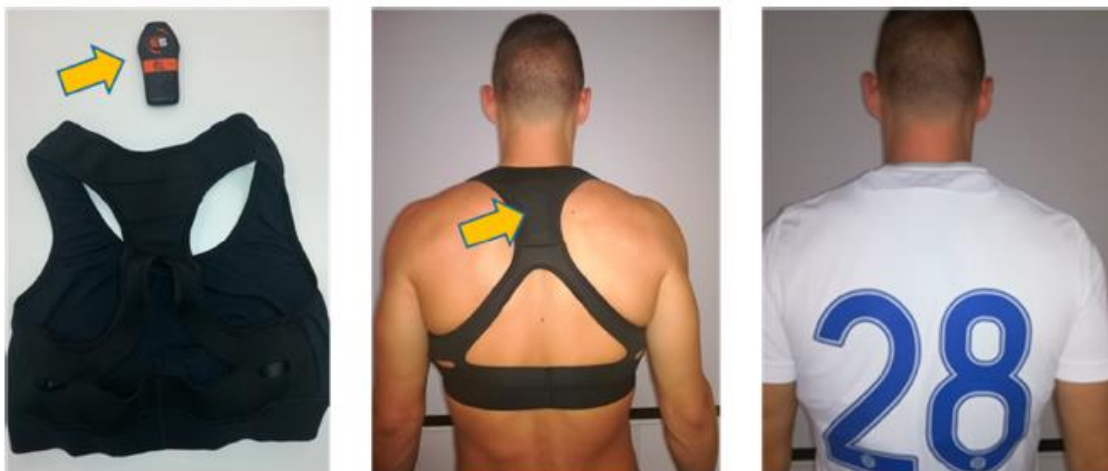
Figure 1. Global positioning device (GPS) used for the measurement of running performances in soccer.
